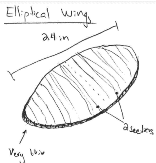
Figure 26 - Elliptical wing design.
