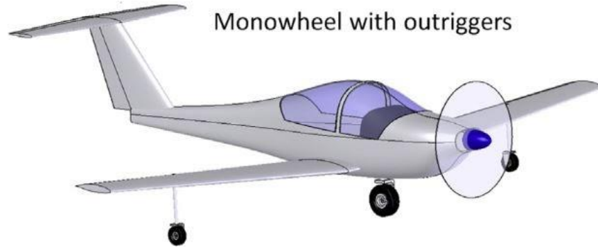
Figure 8 - Monowheel with outrigger landing gear configuration [10].
