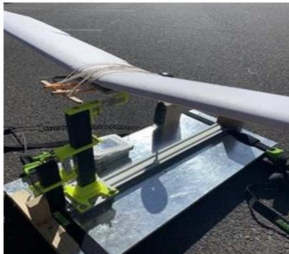
Figure 38 - Lift/drag test stand with wing attached.
