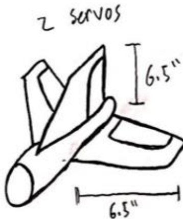
Figure 29 - Conventional tail design.
