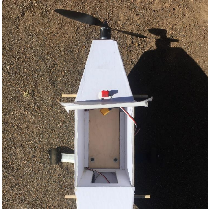
Figure 35 - Photograph of the cargo hold access added to the fuselage.
