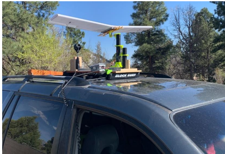
Figure 39- Lift/drag test stand set up on car.
