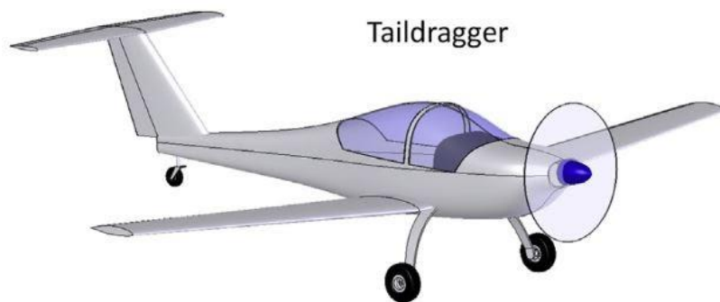
Figure 6 - Taildragger landing gear configuration [10].
